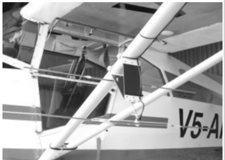
Radio-tracking aerial fitted to the wing strut of the AfriCat Maule.
